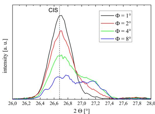
Figure 3: GI-XRD measurement of the Cu(In<sub>1-x</sub>,Ga<sub>x</sub>)Se<sub>2</sub> (112) plane for different incident angles  $\Phi$ . Information depth increases with  $\Phi$ .
