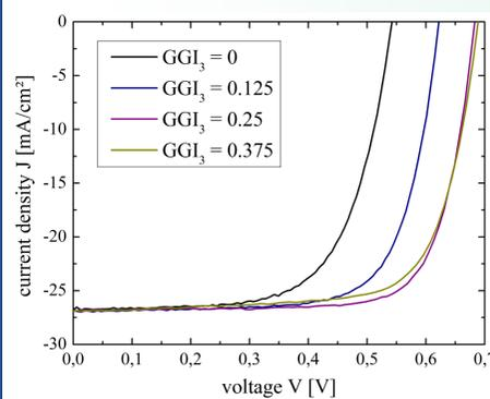
Figure 5: STC current voltage characteristics for the best cell of each absorber type.  $J_{sc}$  might be distorted by slightly different cell sizes.
