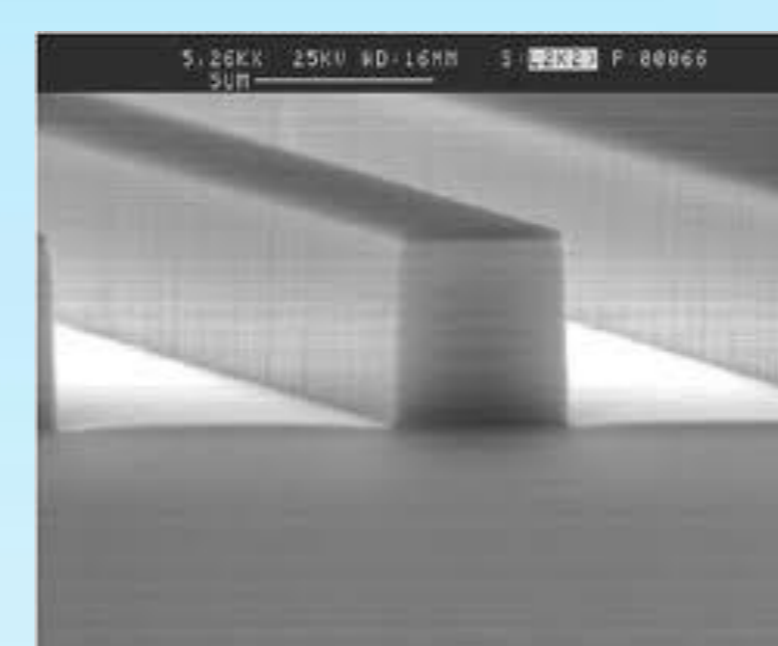
Wave Guide: a wave InP/air
